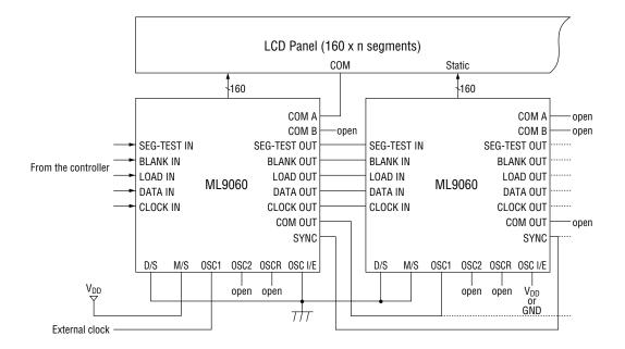
Note: Take care about the resistance and capacitance of wiring for cascade connection.
