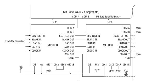
Note: Take care about the resistance and capacitance of wiring for cascade connection.
