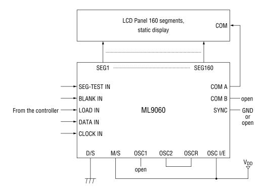
When a single ML9060 is used - 1/2 duty dynamic display mode (external Rf oscillation mode)
